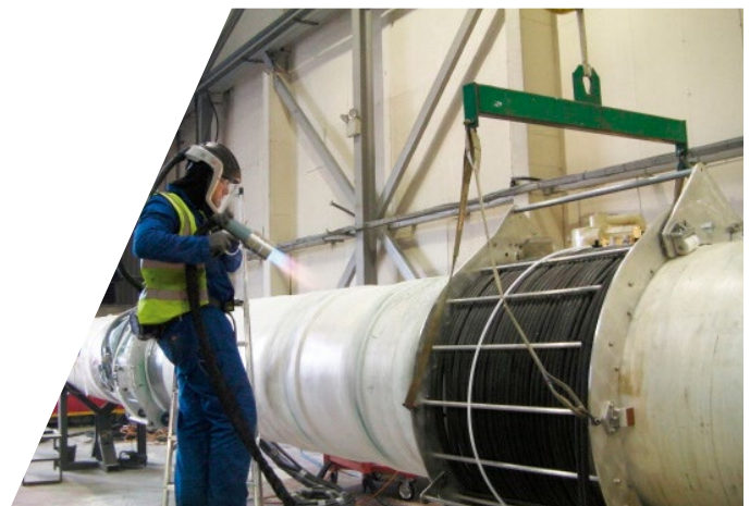
The above field joint is being flame spray coated with Plascoat® PP10.
