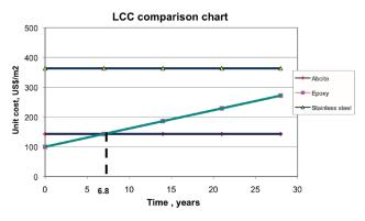
**Figure 1.** Lifecycle costs (LCC) – a comparison between stainless steel, epoxy and thermoplastic (Abcite). Image courtesy of Van Os-Duracoat, Belgium.
