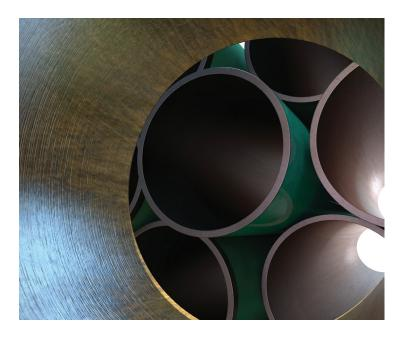
Products in the 7-2500 Series family are typically applied to a hot substrate, ranging from 225°C (438°F) to 239°C (463°F) and cured with residual heat. These coatings can be applied by flocking, fluidized bed or electrostatic spay.
