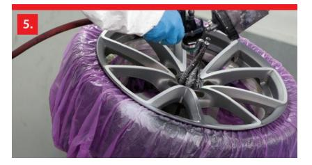
5. To complete the masking process, flip the wheel over, checking that the elasticated band is still creating a seal and then paint.
