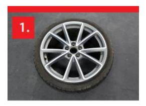
1. Remove wheel from the vehicle and deflate the tire.
