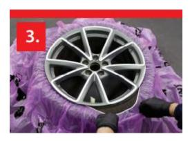
3. Apply the product by placing the elasticated band around the rim, ensuring the treated side of the film is facing upwards.
