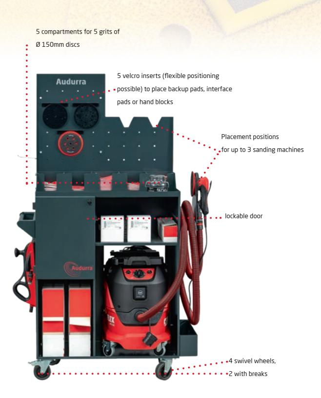
The illustration shows the cart with Audurra products, which are not included in the scope of delivery of the cart,
