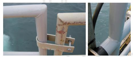
Both rails coated six years ago: Plascoat PPA 571 on the left hand rail, liquid paint on the right hand rail.
