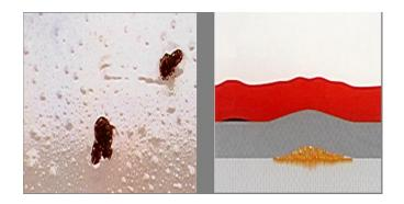
To avoid this type of contamination, the use of solvent-resistant (Nitrile) gloves during panel preparation and handling is recommended, see image 2. This is followed by a cleaning process using lint free wipes with a wax and grease remover to ensure the surface contaminants have been effectively removed from the panel surface before priming.
