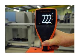
Dry film thickness (DFT) can be measured using two methods:
