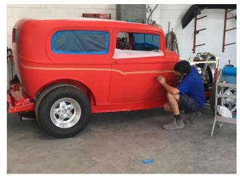
"We stripped it down and sent all the panels off for sandblasting. When they came back, we sealed them up with Cromax 840R Epoxy Primer-Surfacer which has outstanding corrosion resistance and adhesion. Then we did the panel repairs and the filler work and resealed with 840R. Finally, we rubbed it all down and primed it all with Cromax 1040R High-Solids Surfacer."
