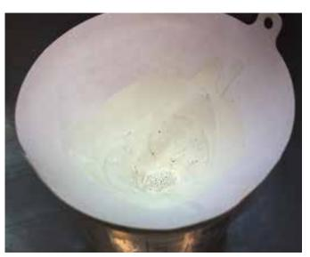
An example of improperly stirred paint – the black pigment has separated and caught in the filter
