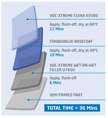
This is an example of the time taken to paint a new OEM primed part using the Standox Xtreme System, which is based on Axalta's Fast-Cure Low-Energy technology.
